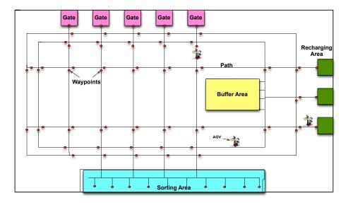
Figure 1: Typical configuration of a warehouse.
