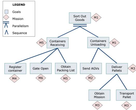
**Fig. 5.** The functional specification of the production groups represented by a goal and mission decomposition tree.
