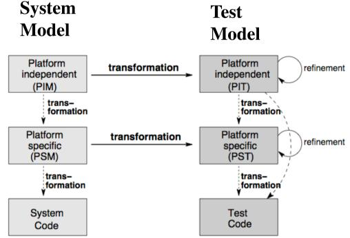
Model-driven testing enables the early integration of testing into the system development process.
