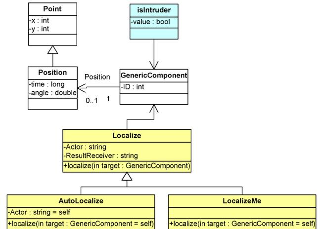
**Figure 3. An example of Domain Ontology Diagram (DOD) representing part of the ontology of a robotics application**
