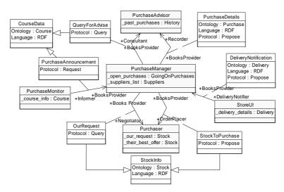
Figure 8. The Communication Ontology diagram
