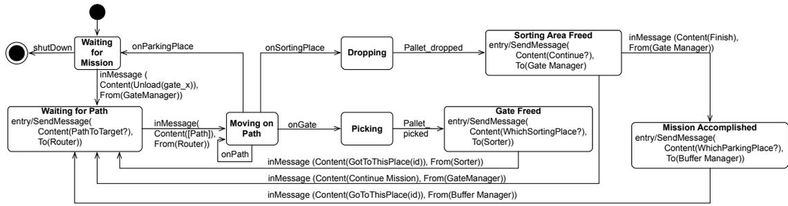
Figure 4: Behavioral model of the Agv's role.
