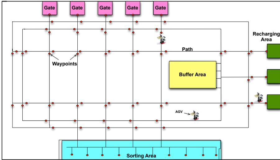
Figure 1: Typical configuration of a warehouse.
