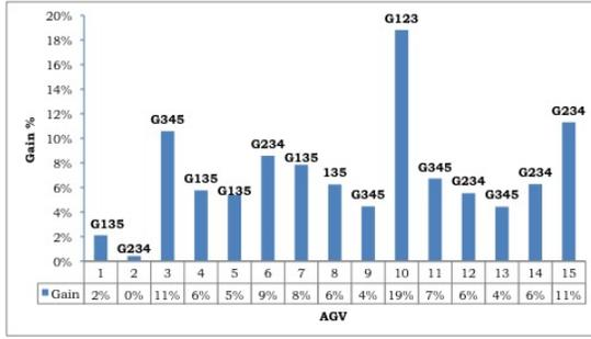
Figure 17: Percentage throughput with the best gate configurations when varying the number of AGVs.
