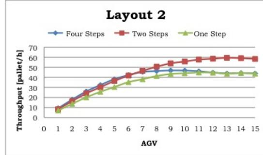
Figure 14: Throughput with different path reservation strategies in a warehouse using *layout 2*.
