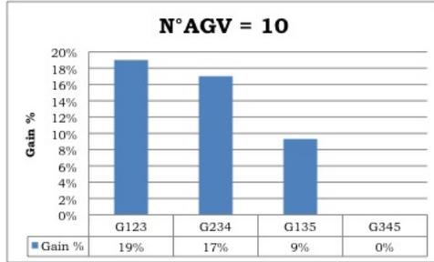
(a) Gain in productivity with different gate configurations.
