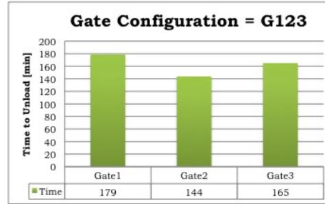
(b) Time required to unload each gate under the most profitable gate configuration (G123).
