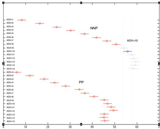
Figure 15: Multiple comparisons test of the effects of different unloading policies and numbers of AGVs on the throughput.
