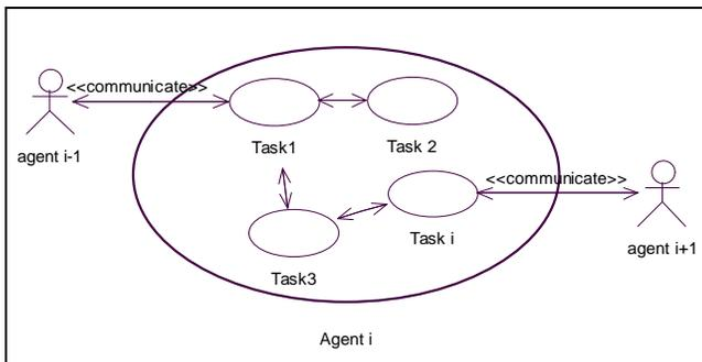
Fig. 2 The internal structure of the agent.
