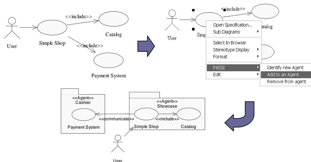
**Figure 2. Three different phases of a toy system design. Up on the left the Domain Description with three use cases, on the right the agent identification phase with the *PTK* context menu and finally down the resulting A.Id. diagram**
