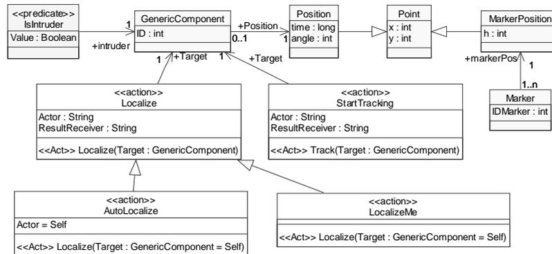
**Figure 3. An example of Domain Ontology Diagram (DOD) representing part of the ontology of a robotics application**
