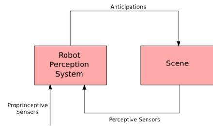
Figure 2: The Robot Perception Loop - redrawn from (Chella and Macaluso 2009)
