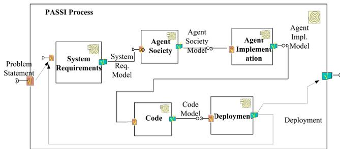
Figure 1: The PASSI Design Process
