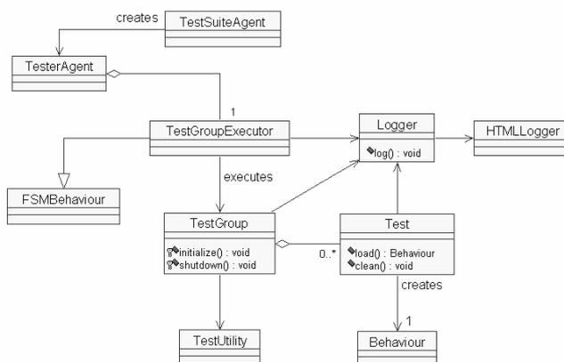
**Figure 3 - Testing framework main classes**
