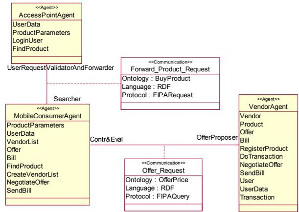
Figure 8: A portion of the COD diagram
