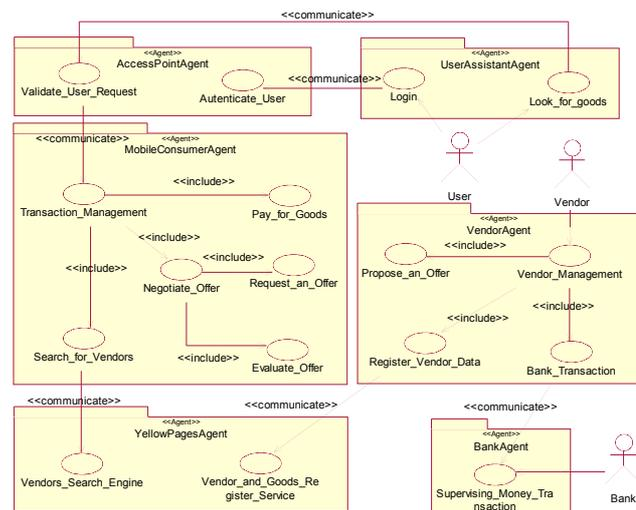
Figure 4: The AId diagram for the proposed case study
