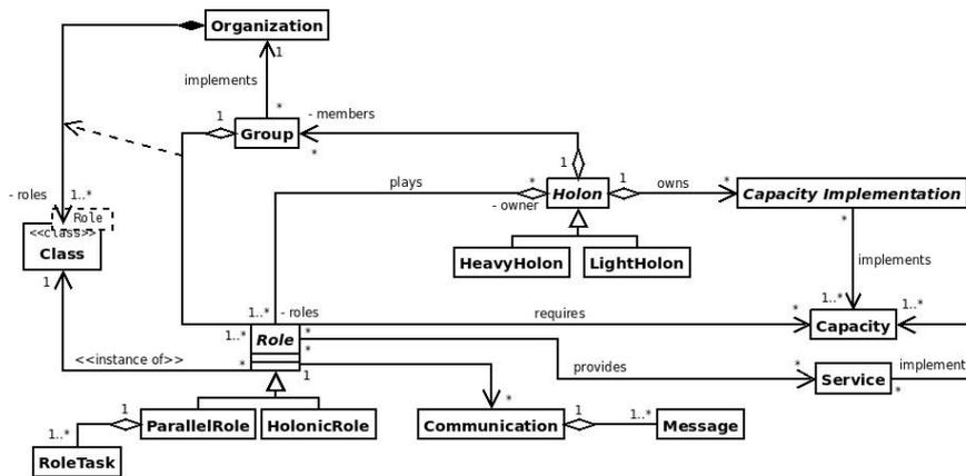
Fig. 5 The UML diagram of the ASPECS metamodel Solution Domain
