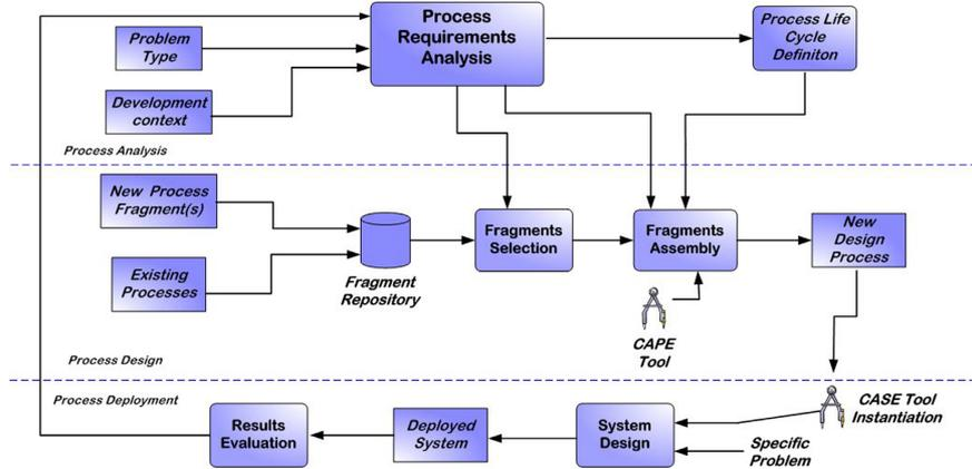
Fig. 1. The PRODE approach for design process composition
