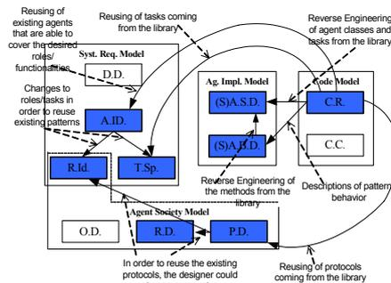
Fig. 5. The resource perspective in the PASSI methodology
