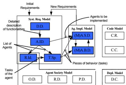
Fig. 2. The architectural perspective in the PASSI methodology
