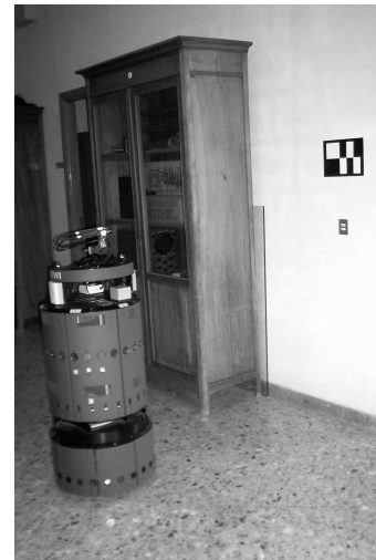
Figure 4: The B21 robot, during a surveillance mission, is calculating its position using the a-priori known position of the marker that it found on its left.
