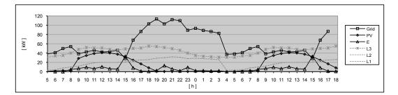
Fig. 3. The power produced by the sources and provided to loads (L1 and L2 curves overlap each other)
