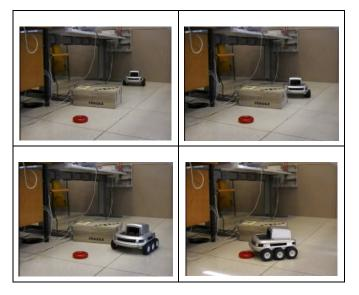
Fig. 5. Some frames of the experimental sequence: Koala robot avoids the obstacle (the box) and reaches the target (red toy).
