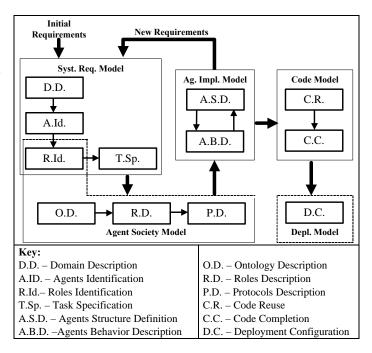
Fig. 3 The models and phases of the PASSI methodology.
