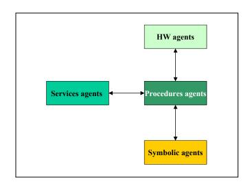
Fig. 4. The proposed multilevel architecture is based on various agents grouped in classes which have different level of knowledge: low level (HW agents), sub-symbolic level (Procedure agents and Services agents), high level (Symbolic agent).
