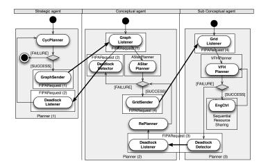
Figure 12: Multi Agent Behaviour Diagram (MABD) for the planning navigation subsystem.
