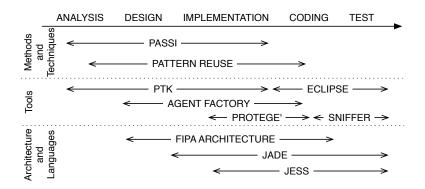
Figure 2: Overview of the framework for the development of robotic multi-agent systems.
