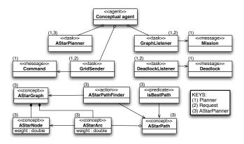
Figure 11: Single Agent Structure Diagram (SASD) for the SLPlanner agent. This PASSI diagram shows how patterns selected for this agent affect the final result. Numeric labels placed near classes indicate the application of more than one design patterns. When more patterns affect the same element, a composition is required.
