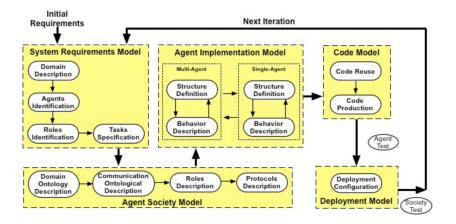
Figure 3: The PASSI design process life-cycle
