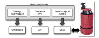
Figure 1: Architectural view of the robotic navigation system
