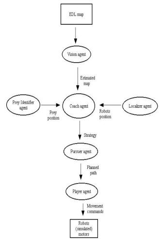
Figure 10: the architecture of our example
