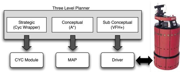
Figure 1: Architectural view of the robotic navigation system
