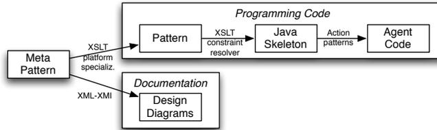
Figure 5: Representation of the pattern code/documentation generation process
